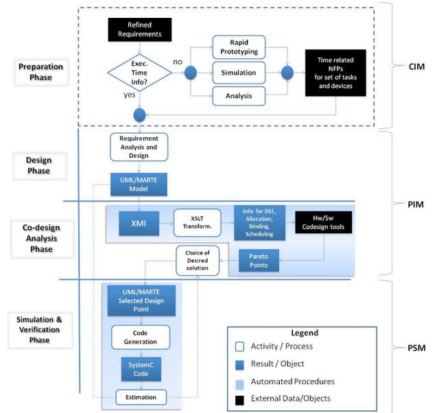
Fig. 2. Semi-automated Design Work-flow.
