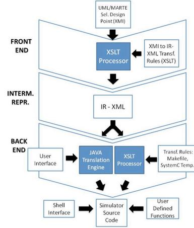
Fig. 3. Automatic Code Generation Procedure.
