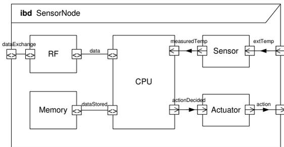
**Figure 2. Internal Block Diagram of the Sensor Node**
