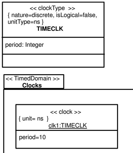
**Figure 3. MARTE representation of a 100MHz Clock**
