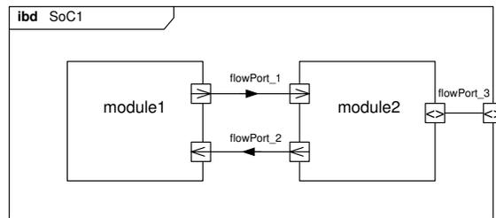
**Figure 1. Internal Block Diagram representing the usage of parts within block SoC1**
